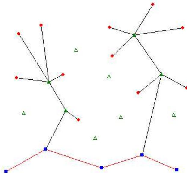
Figure 6.5: Each house connects to the closest node of the minimum spanning tree. Once the 4 transformers are specified this solution becomes the cheapest way to expand the network.
