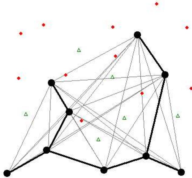
Figure 6.4: The minimum spanning tree of the graph is shown with a thick line.
