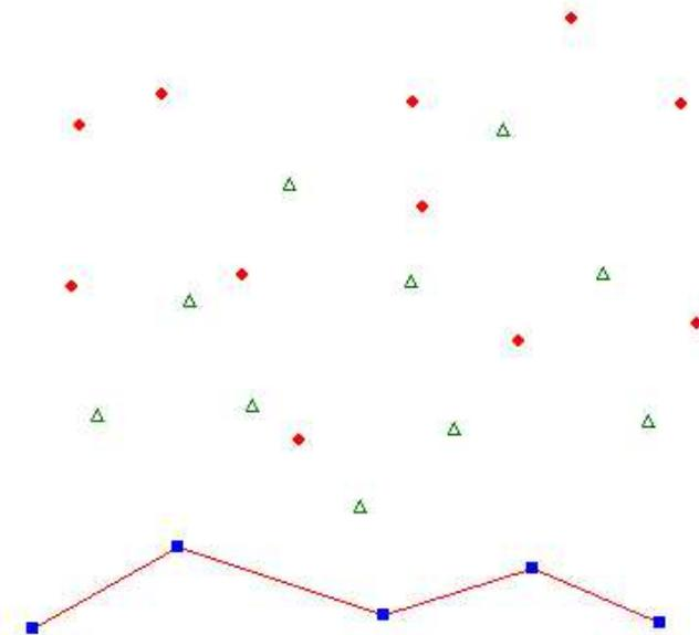
Figure 6.1: The substations, houses, and transformers, are represented by squares, circles, and triangles respectively. In the example there are 5 substations, 11 houses, and 10 possible locations to build transformers.
