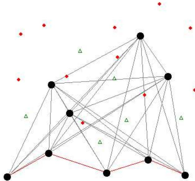
Figure 6.3: An artificial graph is constructed by adding edges from every selected transformer to all the existing substations and to all the other selected transformers.
